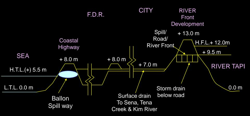
Sketch showing the sectional details for proposed Integrated planning with Coastal Highway & Flood Detention Reservoir
